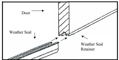
Step 4 Cut off excess weather seal flush leaving two extra inches from the edge of door. Tuck extra weather seal into itself to allow for future shrinkage. If any screws were removed, replace now.
