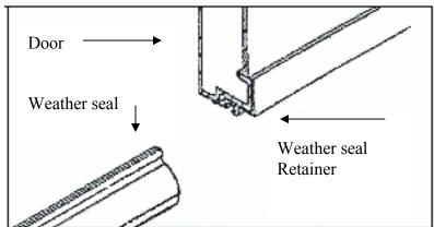
Step 5 Cut off excess weather seal flush leaving two extra inches from the edge of door. Tuck extra weather seal into itself to allow for future shrinkage. If any screws were removed, replace now.
