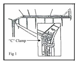
Step 1 Raise door to open position. Place "C" clamps in both tracks directly below the door and tighten. See Fig 1.
